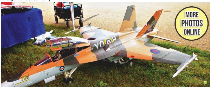
smaller, they burn jet fuel, and their engines can run at the same high speeds as a regular full-sized aircraft.
